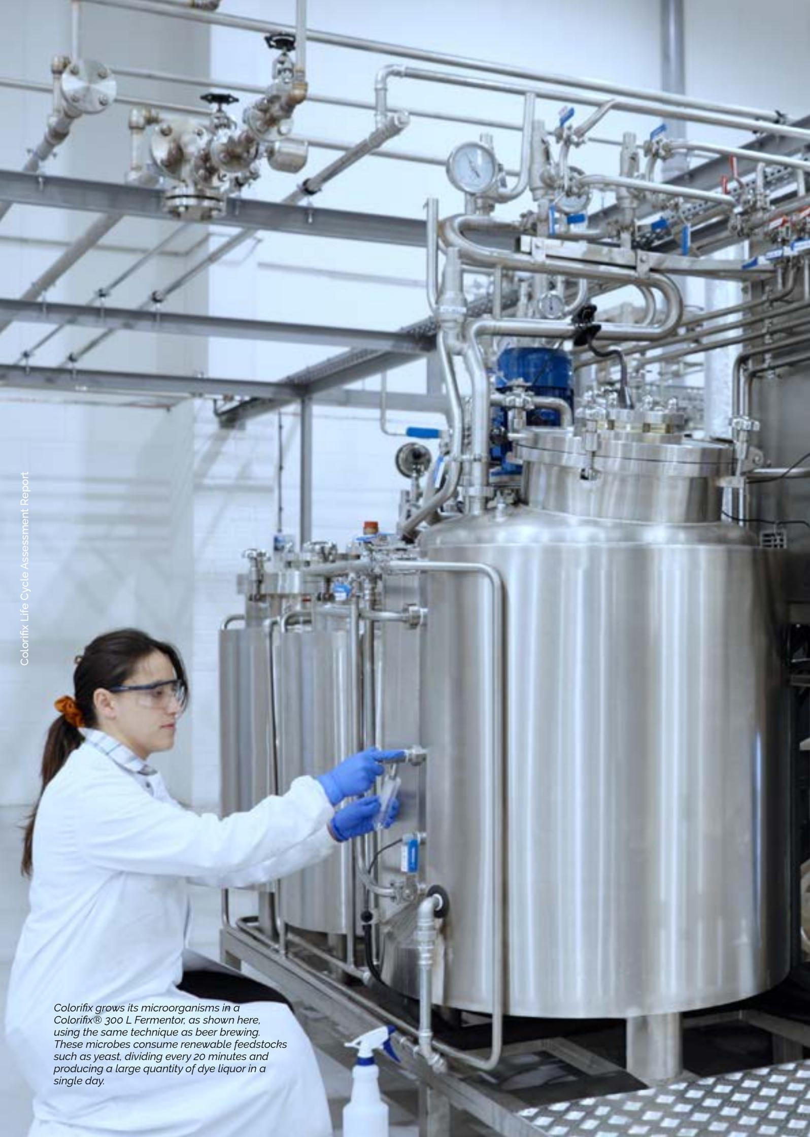
*Colorifix grows its microorganisms in a Colorifix® 300 L Fermentor, as shown here, using the same technique as beer brewing. These microbes consume renewable feedstocks such as yeast, dividing every 20 minutes and producing a large quantity of dye liquor in a single day.*
